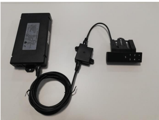
Controller – Bluetooth module – PRO panel
