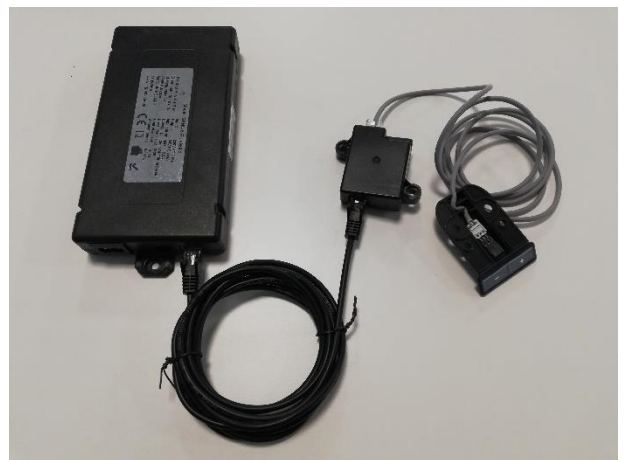
Controller – Bluetooth module – Basic panel
